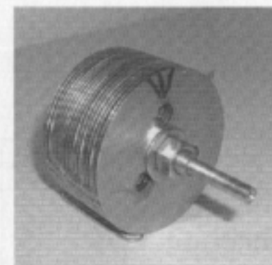
Figure 13. The completed rotor assembly. The diameter has been reduced to 2.70" and the alignment tool has been removed. Note that all exhaust holes remain in alignment.
