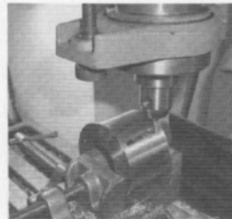
Figure 42. Milling one of the 3/16 " slots in the stator wall.
